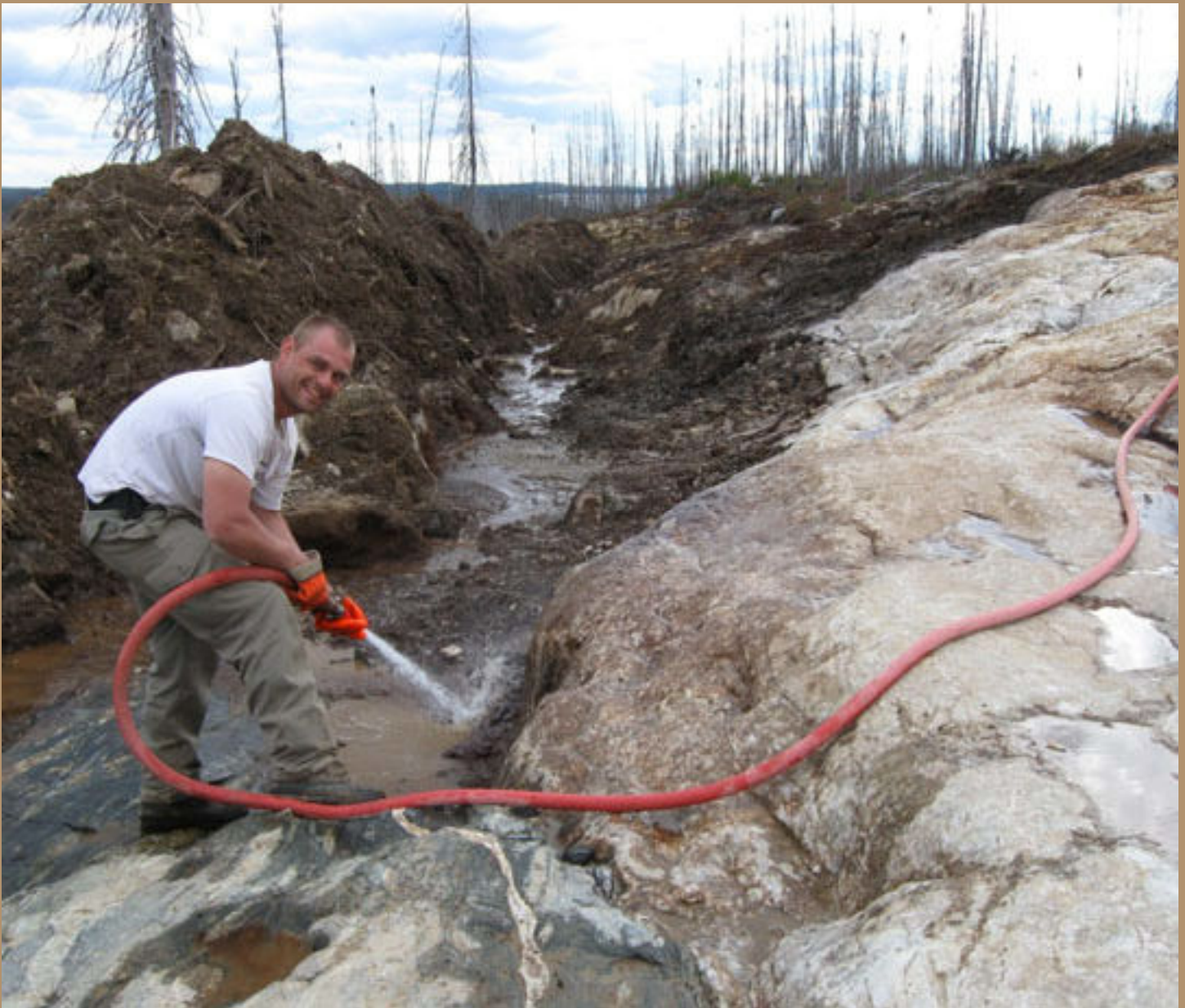
Washing away the overburden from a section of the Whabouchi deposit in preparation for core drilling. Snags in background the result of a previous forest fire.
